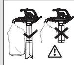
Use only with fully installed suction tube and covered collection bag in suction mode.
