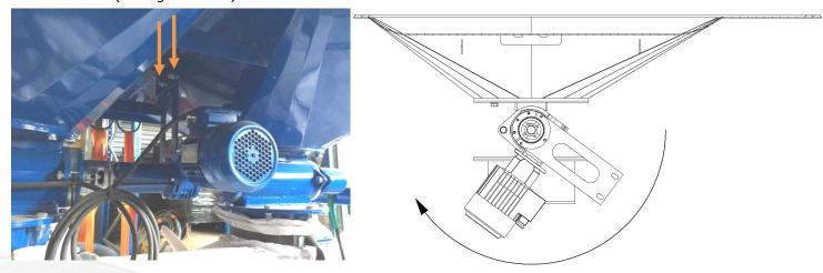
3) Pull out the main plug and remove the bolts and clamp strip of the rotating valve blade.
