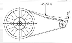
When the belt can be pressed in by hand 5 - 10mm, it has the correct tension. (At  $\pm$ /-  $\pm$ 10 kg pressure)
