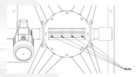
4) Place the new blade and clamp strip and bolts. Apply Loctite 243 on the bolts. First tighten the two inside bolts, than tighten the two outside bolts. Make sure that the seal is in one line with the valve housing and check that the seal has a minimum clearance with the valve housing.
