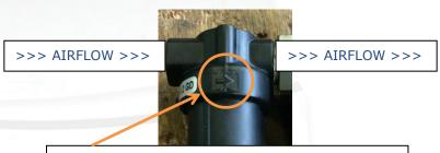
Notice the arrow on the water separator, showing the correct airflow.
