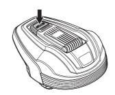
The control panel on the top of the robotic lawnmower is where you manage all the robotic lawnmower settings. Open the control panel cover by pressing down the **STOP** button.
