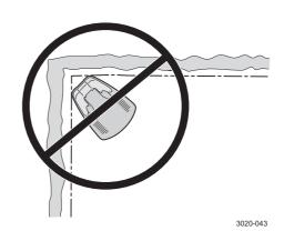
The charging station must be positioned on relatively level ground. The front end of the charging station must be a maximum of 3 cm higher than the back end. The front end of the charging station must never be lower than the back end.
