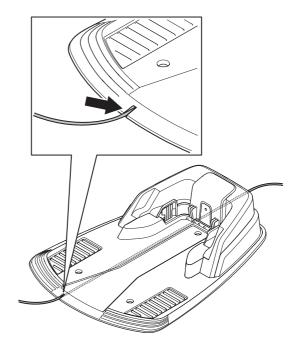
2. Fit the connector to the guide wire in the same way as for the boundary wire described in 3.5 Connecting the boundary wire on page 28. Connect it to the contact pin on the charging station that is labelled "Guide".
