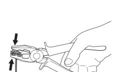
3. Cut off any excess boundary wire 1 or 2 centimetres above each connector.
