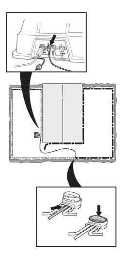
In that case, move the connection for the new wire closer to the disconnected end (roughly at the middle of the suspected wire section) and check again if the indicator lamp is green or flashes yellow.
