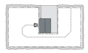
Do not put the charging station in confined spaces in the working area. There must be a straight boundary wire, at least 1.5 metres long, to the right and left of the charging station. The wire must be laid straight out from the rear end of the charging station. Any other locations can mean that the robotic lawnmower enters the charging station sideways and will have difficulty docking.
