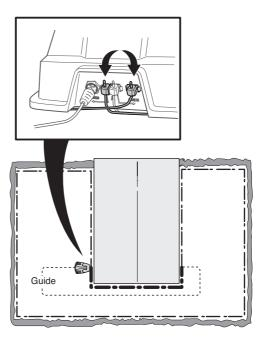
4. a) Assume that the indicator lamp flashed yellow in test a) above. Reset all connections to their original positions. Then disconnect A2. Connect a new loop wire to A2. Connect the other end of this new loop wire somewhere at the centre of the installation.
