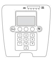
When the stop button has been pressed and the cover is opened, the operation window appears showing the time, selected operating mode, number of mowing hours, battery status and timer setting.
