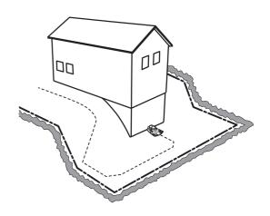
Avoid laying the wire at sharp angles. This can make it difficult for the robotic lawnmower to follow the guide wire.
