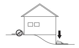
The charging station should not be placed on an island as this limits the laying of the guide wire in an optimal way. If the charging station has to be installed on an island, the guide wire also has to be connected to the island. See the illustration opposite. Read more about islands in chapter 3.4 Installation of the boundary wire on page 22.
