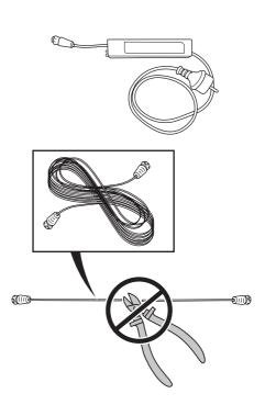
It is possible to let the low voltage cable cross the working area. The low voltage cable must be stapled down or buried, and the cutting height should be such that the blades on the blade disc can never come in contact with the low voltage cable.
