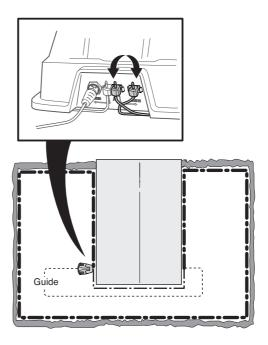
b) Put A1 and Guide back in their original positions. Then switch A2 and Guide. If the indicator lamp flashes yellow, then the break is somewhere on the boundary wire between A2 and the point where the guide wire is connected to the boundary wire (thick black line in the illustration).
