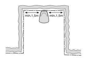
Do not put the charging station in a corner in the working area. There must be a straight boundary wire, at least 1.5 metres long, to the right and left of the charging station.
