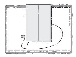
When the break is found, the damaged section must be replaced with a new wire. The damaged section can be cut out if it is possible to shorten the boundary wire. Always use original couplers.
