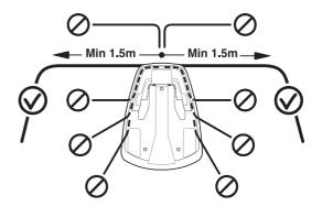
The charging station must be positioned with a great deal of free space in front of it (at least 3 metres). It should also be centrally placed in the working area to make it easier for the robotic lawnmower to reach all areas in the working area.
