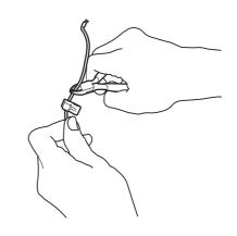
Press the connector onto the metal pin, Press the connector onto the contact pin, marked AL (left) and AR (right), on the charging station.
